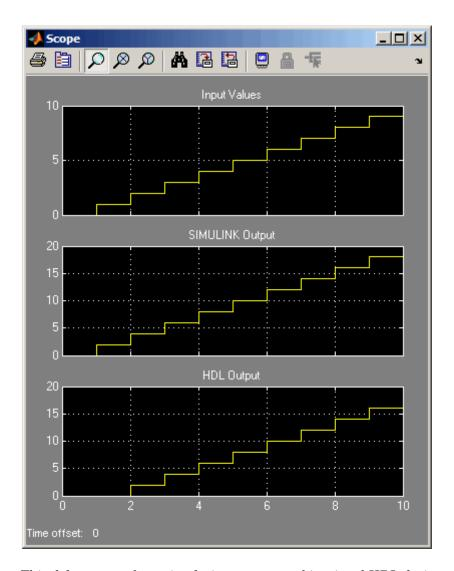
This delay occurs from simulating a pure combinational HDL design without applying direct feedthrough.
