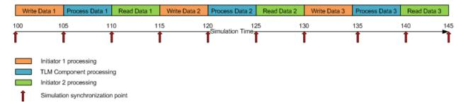
Without temporal decoupling, all the threads execute in sequential order and to exchange the three data the component requires nine context switches.
