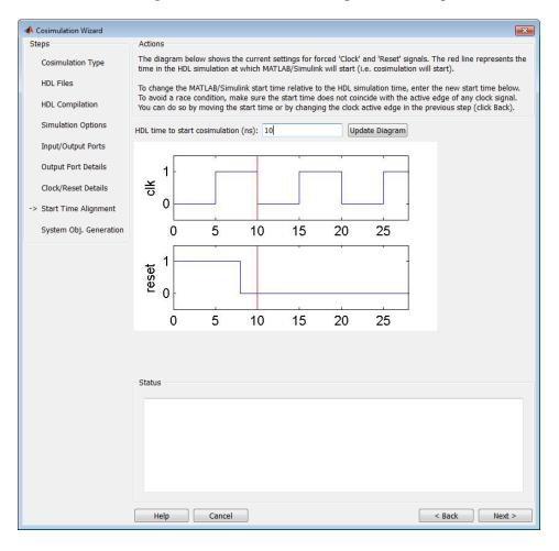
1 In the **Start Time Alignment** pane, review the current settings for clocks and resets. The purpose for this dialog is twofold:
