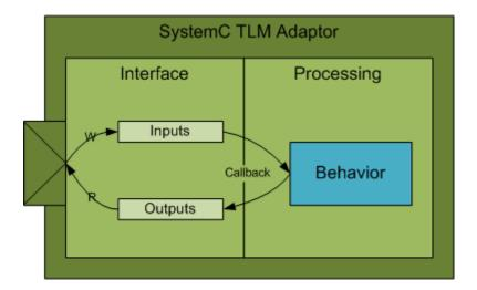
There are a number of options you can use to control the architecture of the generated TLM component. Incorporating a memory map is one of the most effective options. The following figure demonstrates the behavior of a generated TLM component with a full complement of features enabled.
