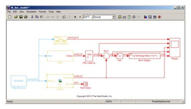
Run simulation. Observe the output waveforms from the behavioral filter block, the FIL block, and the error margin. Because the behavioral filter block does not have pipeline registers, there are small differences between the behavioral filter block output and the FIL block output. These errors are within the error margin.
