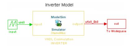
The model contains an HDL Cosimulation block (labeled VHDL Cosimulation INVERTER) simulating an 8-bit inverter that is enabled by an explicit clock. The inverter has a single input and a single output. The following sample shows VHDL code for the inverter:
