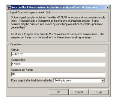
The sample rate and frame size of the input signal propagate throughout the model.
