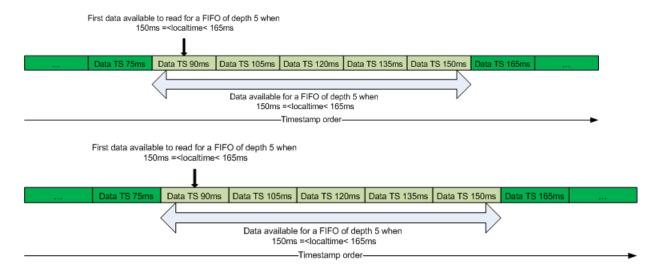
The TLM component also queues all events exchanged between the interface and the processing parts of the TLM component in temporal queues. HDL Verifier generates all timings using a timing annotation to the local time.
